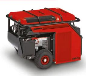
CMP-P10-12 to CMP-P14 is a powerful alternative to electrical tools. Small, compact and lightweight, at only 155kg weight with 1.0 to 1.4 m<sup>3</sup>/min at 7 to 12 bar. Perfect for a wide-range of repair and installation jobs.
